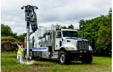
The X-Cavator™ CXT is the legacy Vac-Con hydrovac. This unit was designed with the power and performance expected from Vac-Con machines with a focus on hydroexcavation applications.
