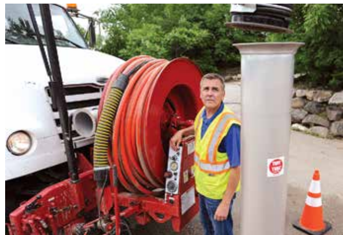
Dave Bogie rotates the vacuum boom on a Vac-Con hydroexcavator to connect an extension tube.
