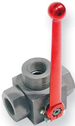
▲ Hycon 1" 3 Way Ball Valve 662-0003 - 2500 PSI
