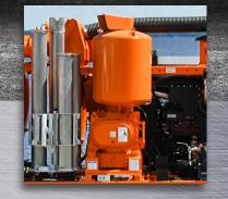
**PD Blower** PD Blower with multiple ratings up to 27" Hg and 5,775 CFM.
